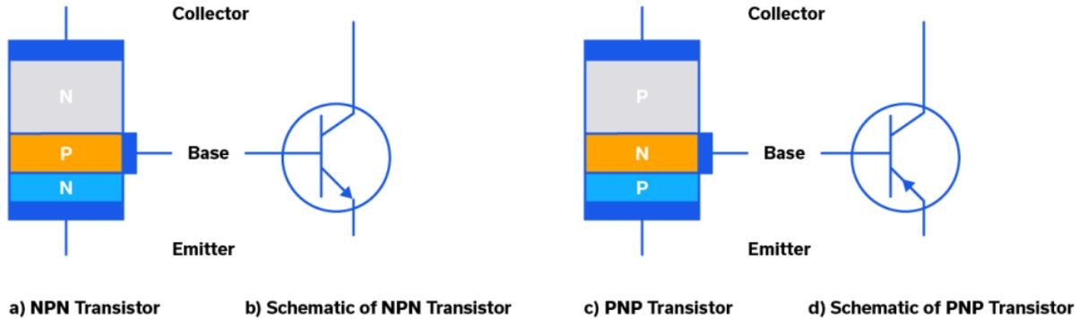
**Figure 1: NPN and PNP transistors.**
