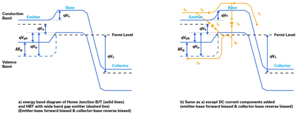
**Figure 5: Energy band diagram, currents; homojunction vs. heterojunction bipolar transistor.**
