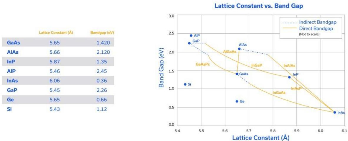
**Figure 4: Lattice constant vs. band gap of various semiconductor materials.**
