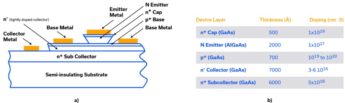
**Figure 6: Typical HBT cross section, layer thickness and doping [12].**
