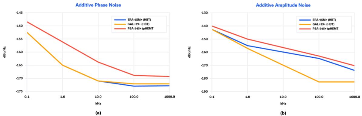
**Figure 8: Additive phase and amplitude noise of HBT and pHEMT amplifiers.**
