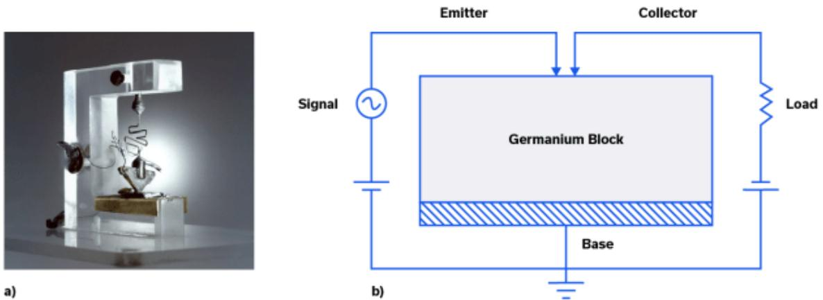
**Figure 3: Original point contact transistor.**
