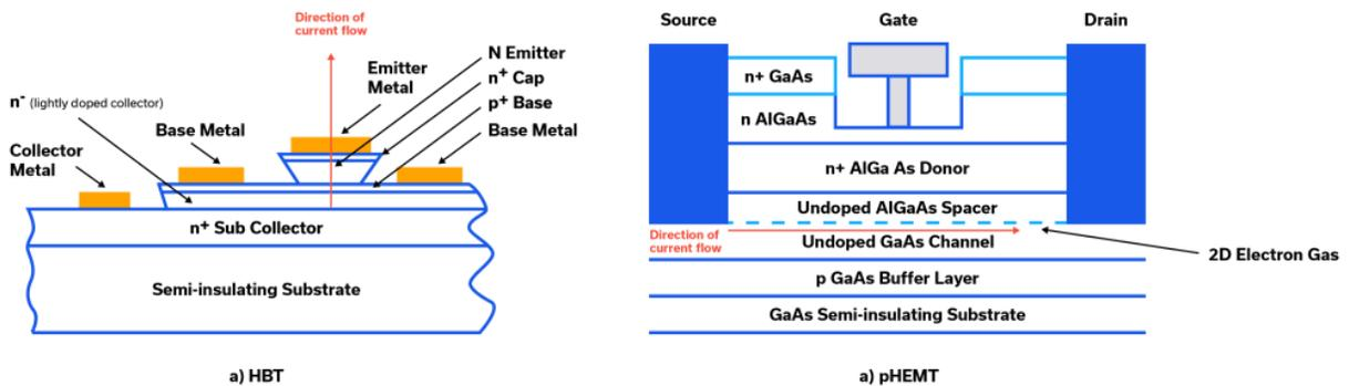
**Figure 7: Direction of current flow in HBT and pHEMT.**
