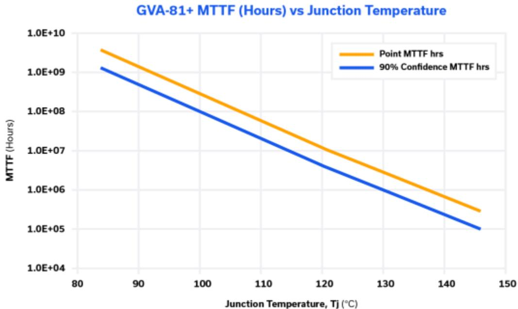
**Figure 9: MTTF vs. junction temperature for GVA-81+ HBT-based MMIC amplifier.**
