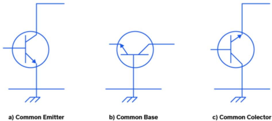
**Figure 2: Biasing configurations for an NPN transistor.**
